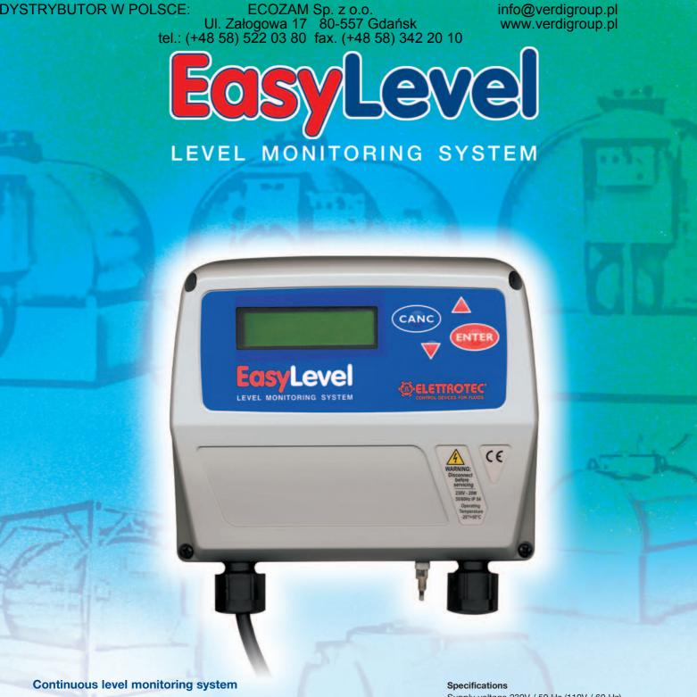
EasyLevel is an innovative system for monitoring the fluid level inside atmospheric tanks. The system detects the static pressure generated by the fluid height by means of a tube inserted in the tank and displays the fluid level or volume. The new design and technology guarantee a reliable and repeated level indication.
